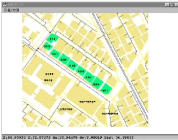
Figure 5. Valves which should be closed and buildings which have possibility of suspension of water supply
