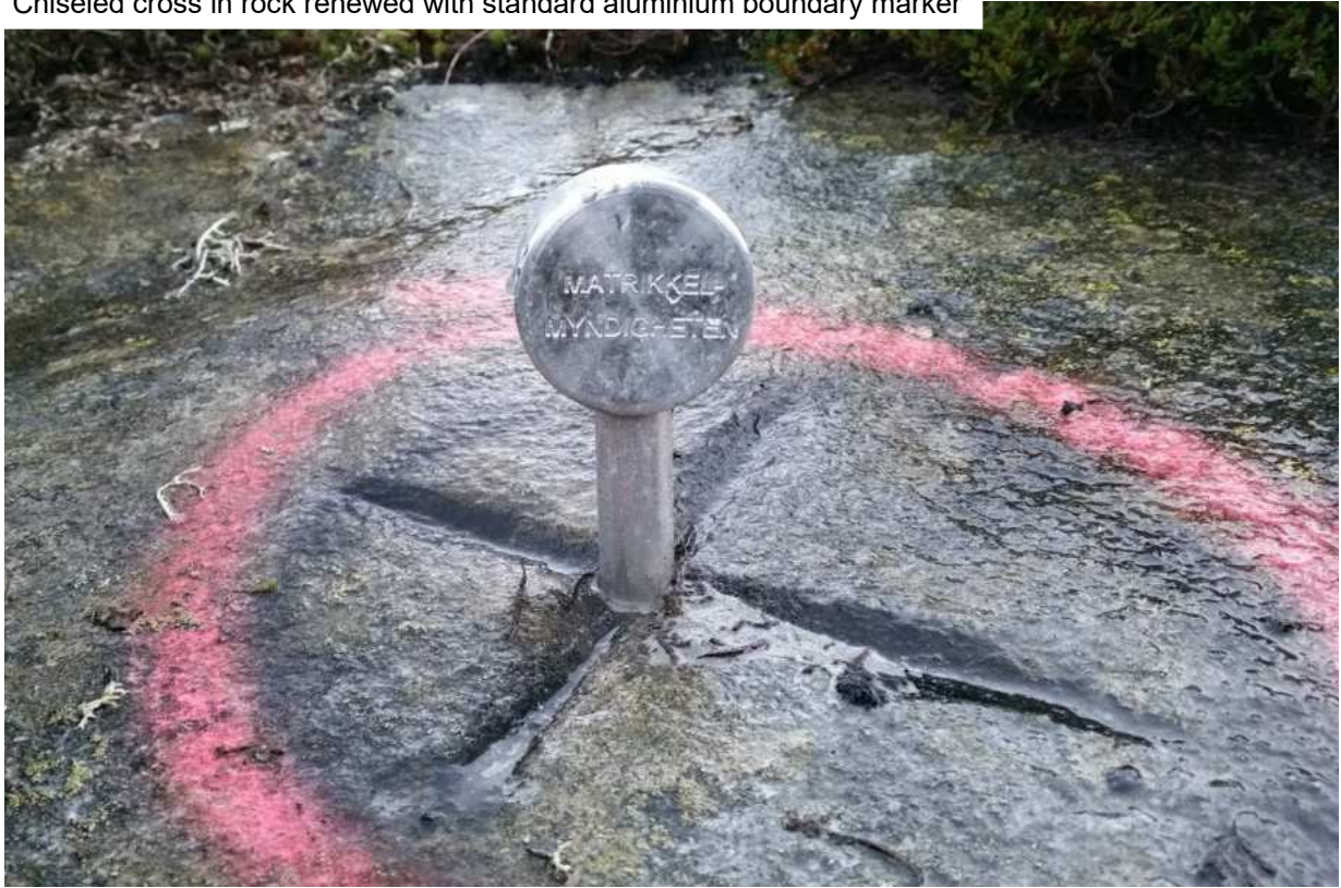
Chiseled cross in rock renewed with standard aluminium boundary marker
