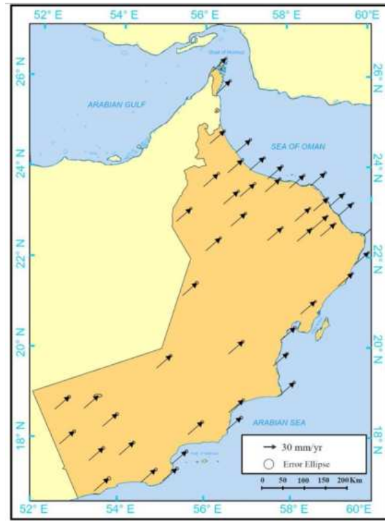
Figure 3: Final horizontal velocity field of OMANCORSNET in ITRF20
