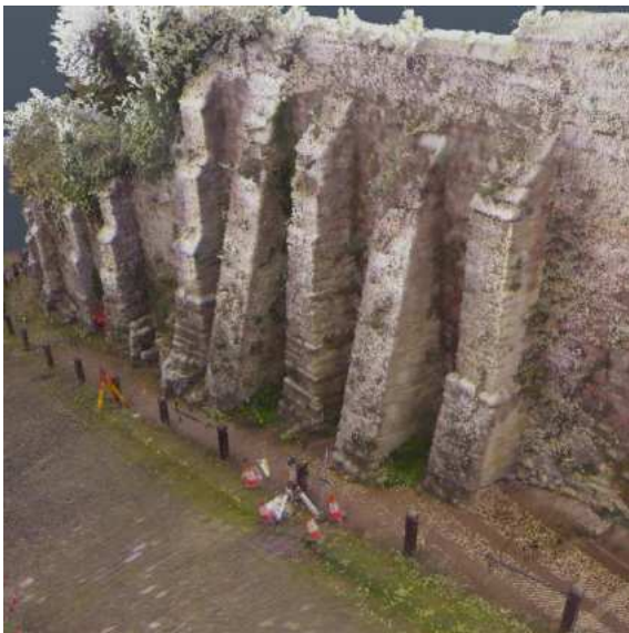
Figures 11 & 12. Final 3-dimensional model of the retaining wall at Gold Hill viewed in Autodesk ReCAP
