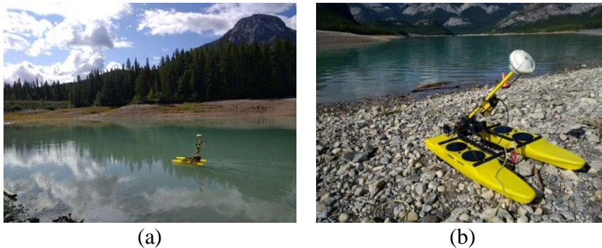
Figure 1. HyDrone performing mapping of a lake bed (a); a close-up of the HyDrone before deploying
