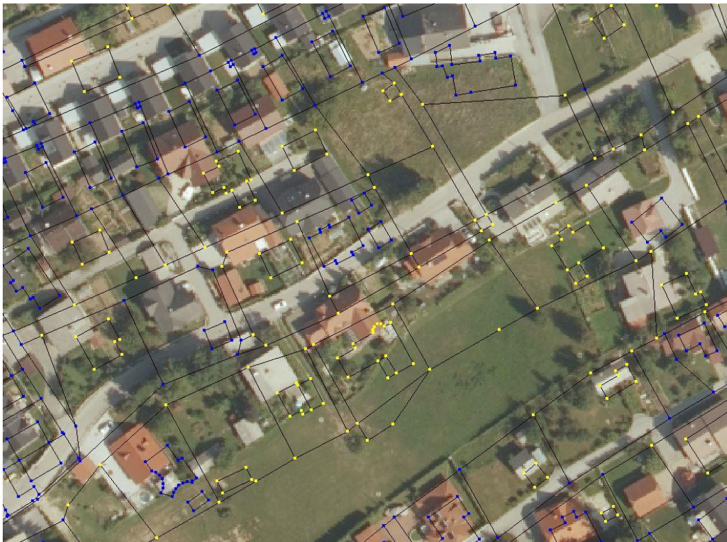
Figure 1: Land cadastre graphical data: – the ZKP ( SysGeoProTM ). KEY: reference (measured) points – blue, subject (digitized) points – yellow, the ZKP lines – black.
