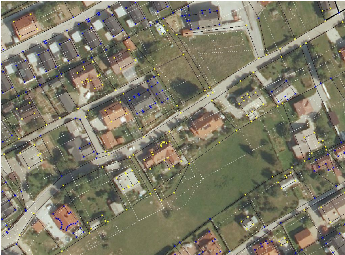
Figure 3: The result of the improved positional accuracy of the ZKP ( SysGeoProTM ). KEY: reference points – blue, digitized points – yellow, ZKP lines before improvement – intermittent white, ZKP lines after improvement – black.
