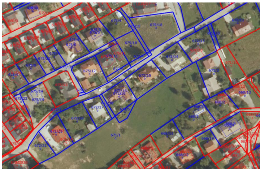
Figure 4: The ZKN after the implemented positional accuracy improvement and ZKP integration, as seen in the public viewer PREG.KEY: The ZKN obtained by measurements – red, the ZKP after positional accuracy improvement – blue.
