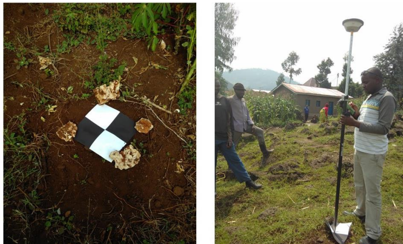
Figure 2: Measurement of ground reference points
