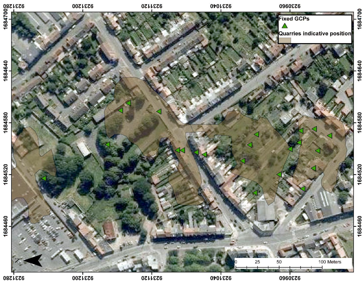
Figure 5. Series of GCPs that have been used for the georeferencing of the point cloud data. Axes represent planimetric coordinates in meters.
