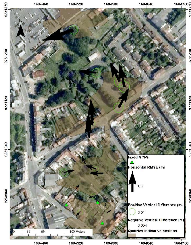
Figure 7. RMSE when only three GCPs are held fixed. Showing significant horizontal error with an increase in range from the held GCPs.
