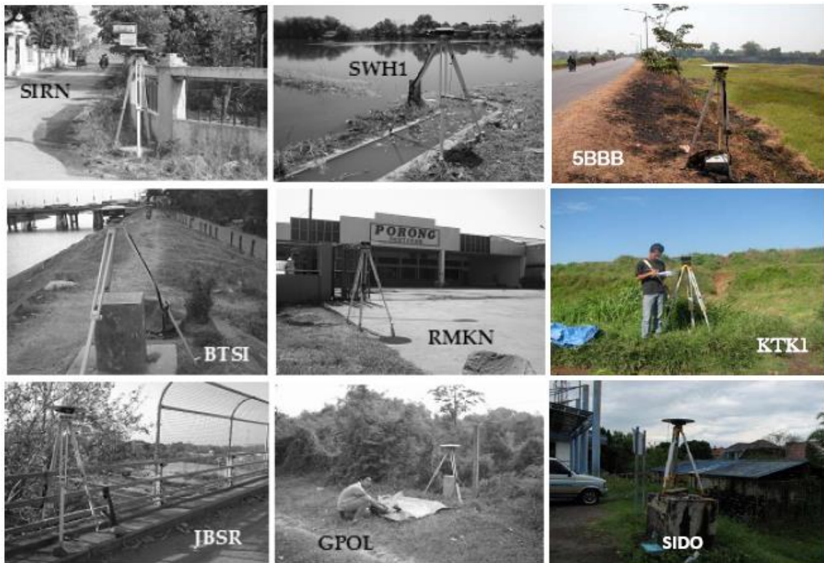
Figure 5 Some documentation of GPS survey in the field using dual-frequency geodetic-type receivers, with observation session length of about 5-10 hours
