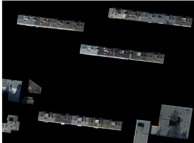
Orthorectified image of set of building roofs
