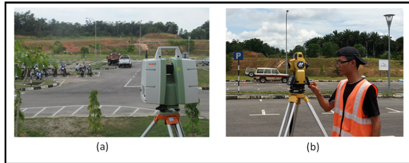
Figure 6: (a) Leica Scan Station C10 is used to scan the land slope surface and (b) reflectorless Total Station Topcon ES-105 is used for validation.
