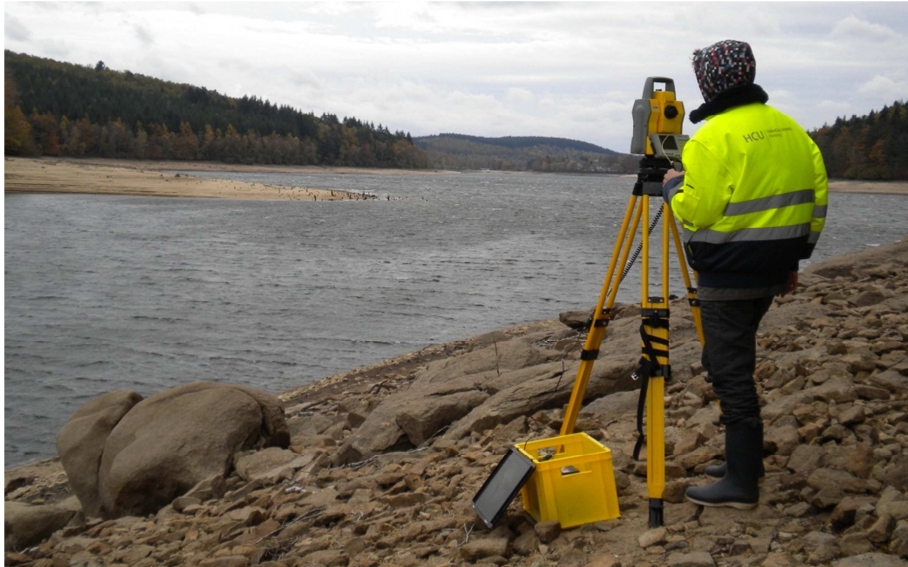
Figure 3: Topographic measurements on the lake shore
