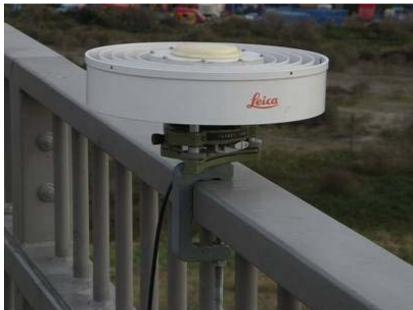
Figure 4. GPS Antenna Set up showing Clamp and Tribrach Attachment
