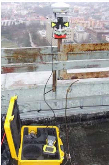
Fig. 2 GNSS antenna and receiver Trimble R8 with prism
