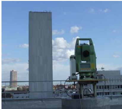
Fig. 1 Robotic UMS Leica TCA 1101 with inclinometers
