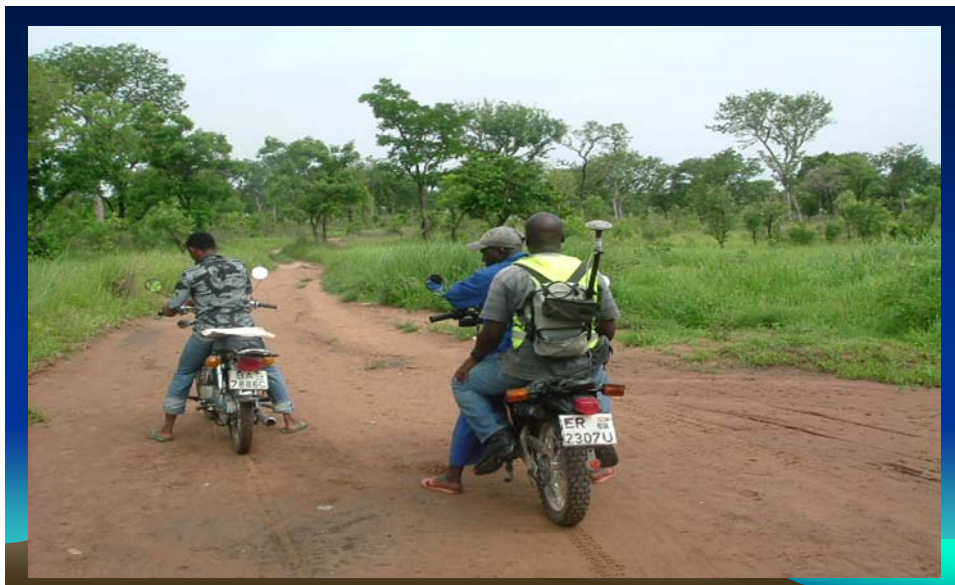
Fig. 4: Survey carried out using a motorbike and bag packed GPS using two axles due to inaccessibility of four wheels
