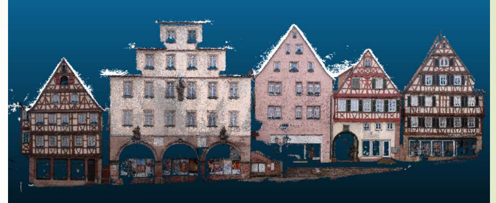
Very dense 3D reconstruction using Absolute Oriented Images
