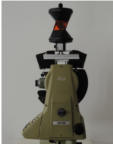
Fig. 1 Measurement setup for prism investigations: adapted Leica TM1100 with rotating 360° prism
