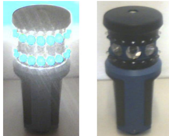
Fig. 16 Trimble MultiTrack (MT) 1000 in active (left) and passive (right) mode. Images captured with an infrared camera
