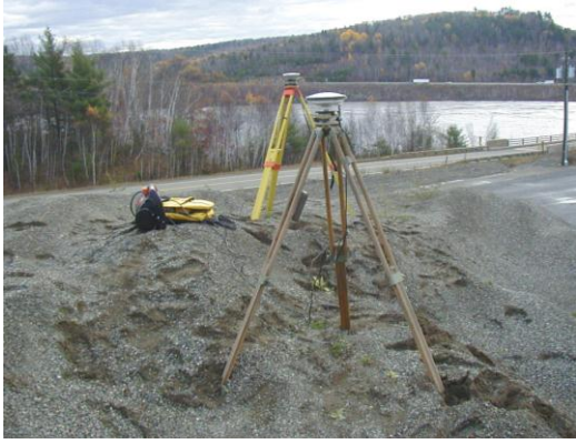
Figure 11. Detail of reference stations used for monitoring the bridge
