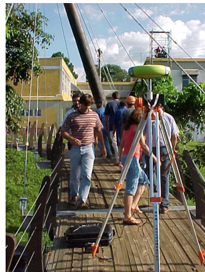
Figure 6. Front view of pedestrians walking on the footbridge and view of the GPS antenna over the oscillator
