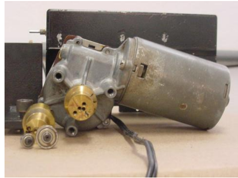
Figure 03. Detail of the electro-mechanical oscillator
