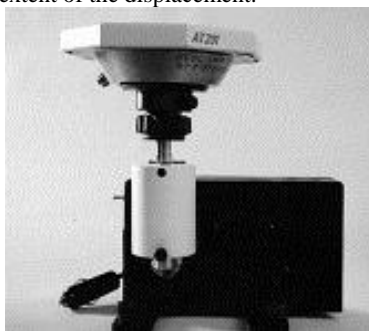
Figure 02. GPS antenna over the electro-mechanical oscillator
