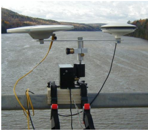
Figure 12. Wooden support for the electro-mechanical device
