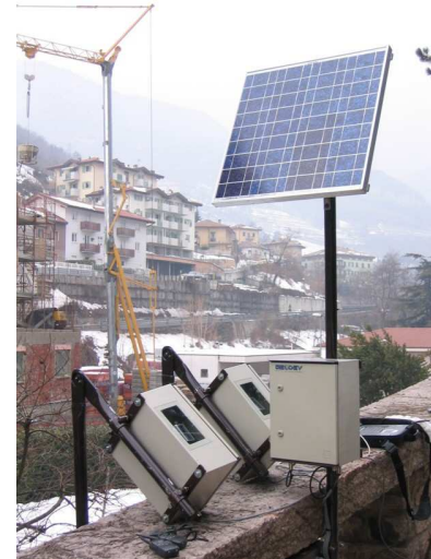
Figure 3 - Installation with two 3DeMoN-Laser instruments and a 3DeMoN Monitoring Station with solar power supply
