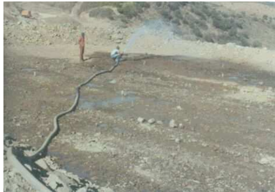
Figure 2 –Beliche Dam. Stage of abundant irrigation in the collapse test
