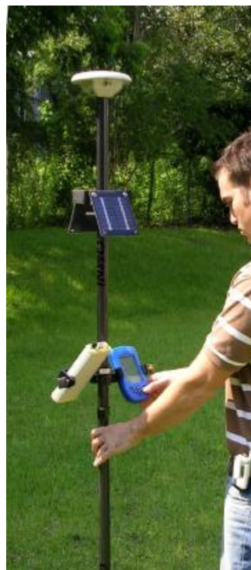
Figure 2. DataGrid Mk-1 Crane or Toughman GPS/Data collectors in typical field configuration. Shown on a pole with low weight antenna, solar panels and a PDA.
