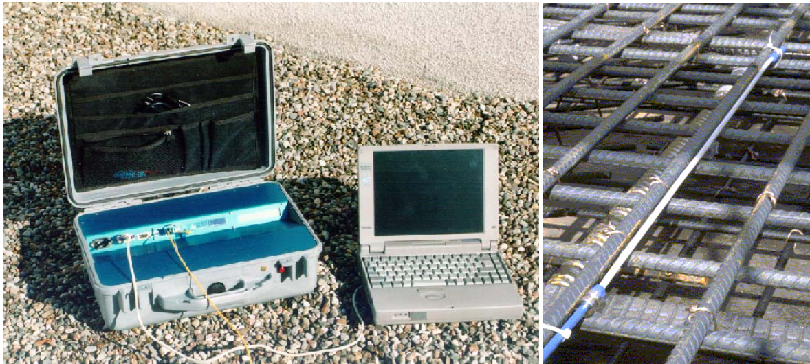
Figure 1: SOFO system reading unit and SOFO sensor installed on a rebar
