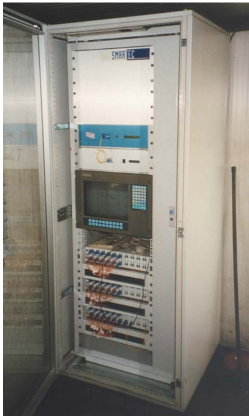
Fig. 3: Setup of the SOFO system used for static measurements.
