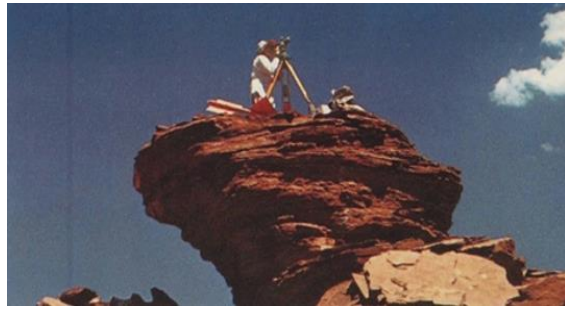
Above: Brad Washburn of National Geographic in 1970 with Wild T3 during the Grand Canyon survey on Dona Butte. In 1983, Washburn also had Swissphoto fly over Mount Everest with a Wild RC10 and in 1987 he had it photogrammetrically restituted and mapped in Switzerland with the stereo plotter Wild A8 by Swisstopo (see map section at bottom left). ((RE))
