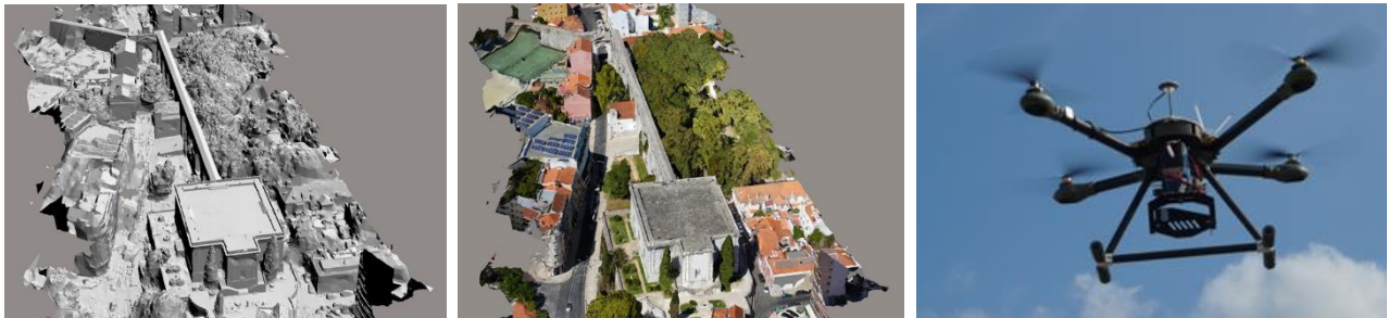
Figure 6 – 3D modelling using UAV collected data for the “Mãe de Água” water reservoir
