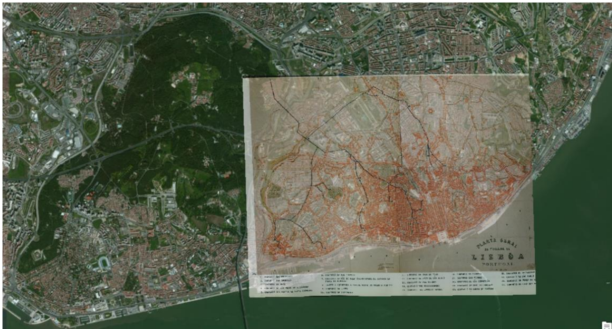
Figure 4 – Identification of the Lisbon Aqueduct System using ancient cartography (Planta Geral da Cidade de Lisboa, 1868), GIS georeferencing (transparent) over satellite imagery
