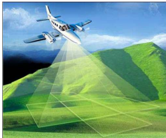
Figure 1, The Pictometry camera sensor systems consists of five cameras, one directed nadir, the others viewing forward, backward, left and right (Image Courtesy: Blom Group).
