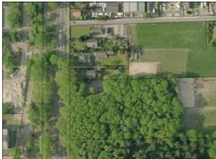
Figure 3, Cadastral map (black lines) superimposed on Pictometry ortho-image.
