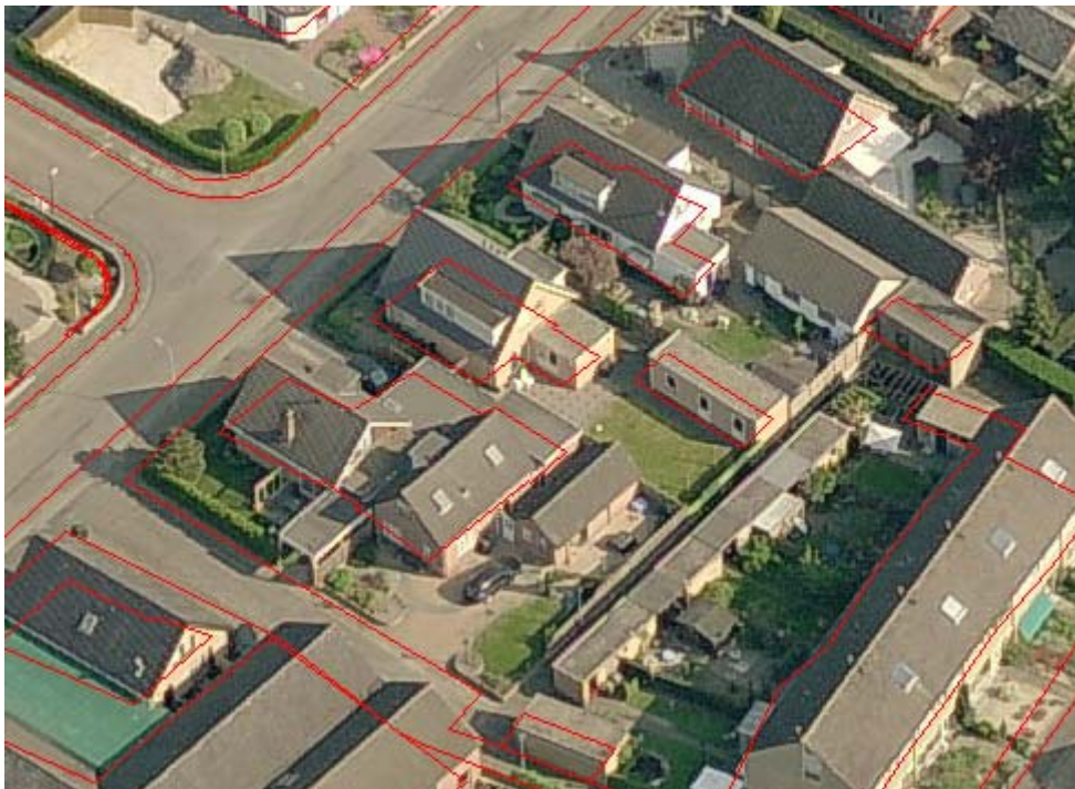
Figure 5, Projection of GBKN lines into oblique image.
