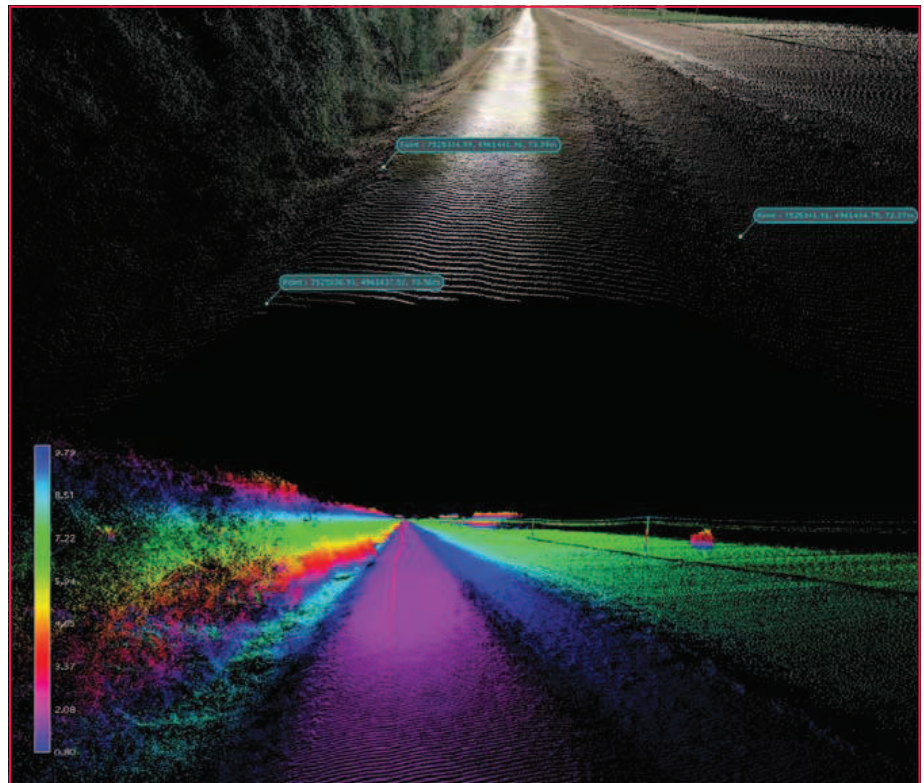
Figure 4: Surveying the river embankment by using mobile laser scanning technology
