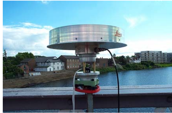
Figure 3: The accelerometer and Leica AT504 choke ring GPS antenna housed together as one unit
