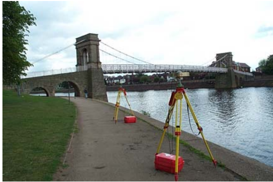
Figure 2: The two riverside reference stations with the Wilford Bridge in the background
