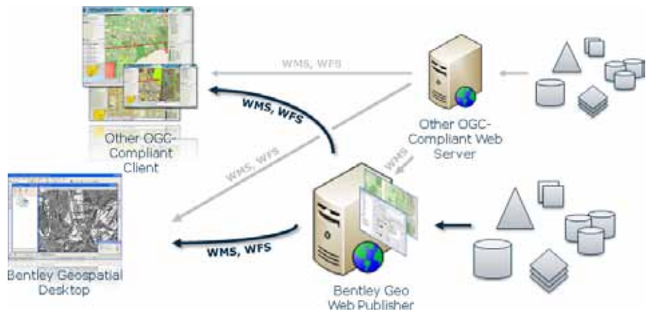
This figure illustrates the publishing of data using OGC's WMS and WFS protocols, serving either Bentley geospatial desktop or other OGC-compliant clients. Note how Bentley Geo Web Publisher services both types of clients and can act as a cascading WMS server, passing on WMS data received from other OGC-compliant web servers.
