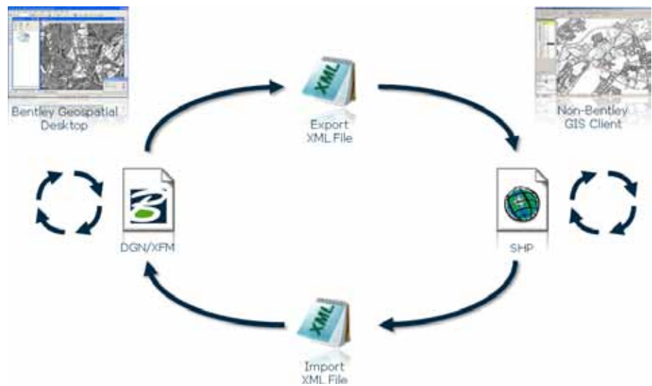
This figure illustrates the data exchange lifecycle between the Bentley geospatial desktop and a non-Bentley GIS client. The lifecycle leverages Bentley's semantic interoperability tools by using import and export XML files to map DGN/XFM objects to SHP data.
